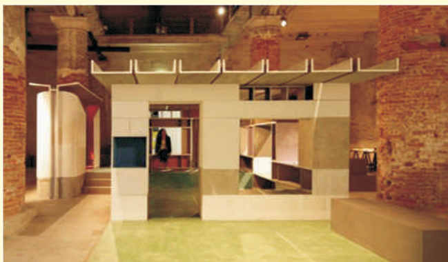
Ferrocement blocks used in this Full Fill Homes model can be produced in the backyards of masons' homes, providing an additional income
